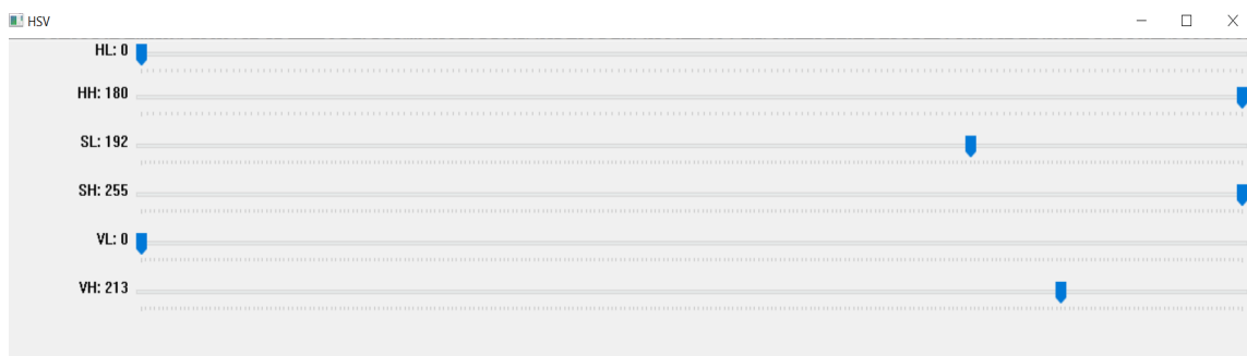
Figure 2.1.1: Tracker to adjust HSV mask parameters
