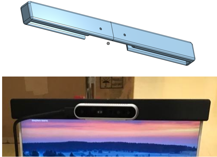
Figure 2.3.3 and 2.3.4: Camera mounting CAD and printed part
